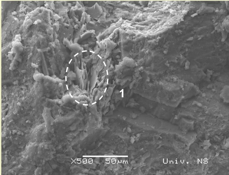
SEM micrograph of the stone sample PTT 10, x500
